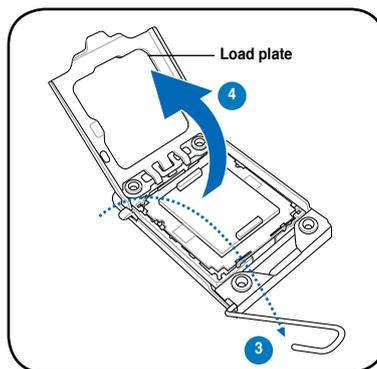
5. Remove the PnP cap from the CPU socket.
