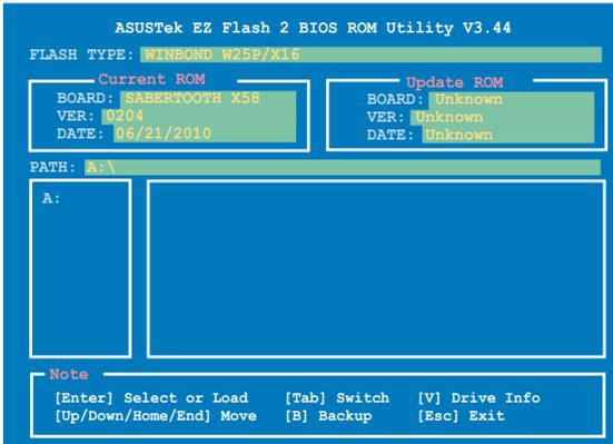
2. Press <Tab> to switch between drives until the correct BIOS file is found. When the correct BIOS file is found, EZ Flash 2 performs the BIOS update process and automatically reboots the system when done.
