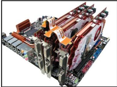
5. Connect three independent auxiliary power sources from the power supply to the three graphics cards separately.
