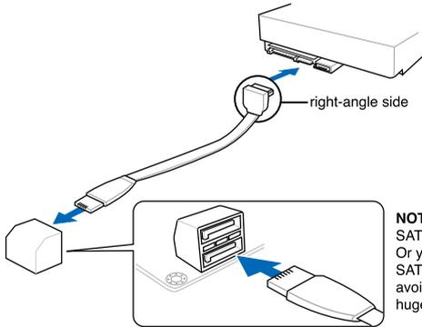
**NOTE:** Connect the right-angle side of SATA signal cable to SATA device. Or you may connect the right-angle side of SATA cable to the onboard SATA port to avoid mechanical conflict with huge graphics cards.
