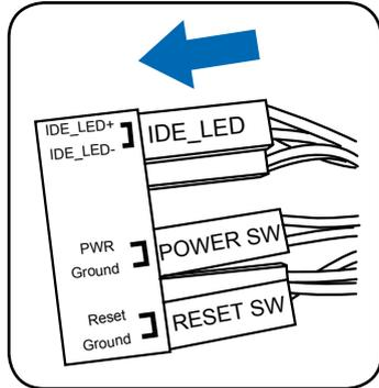
2. Install the ASUS Q-Connector to the system panel connector, ensuring the orientation matches the labels on the motherboard.
