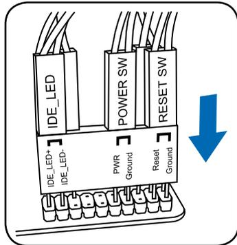
3. The front panel functions are now enabled. The figure shows the Q-Connector is properly installed on the motherboard.
